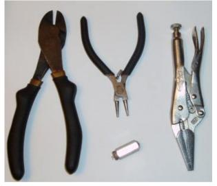
R to L – **Tools** includes diagonal wire cutter, looping, pliers, Du-Bro E/Z Twist and a needle nose Vise Grips.
